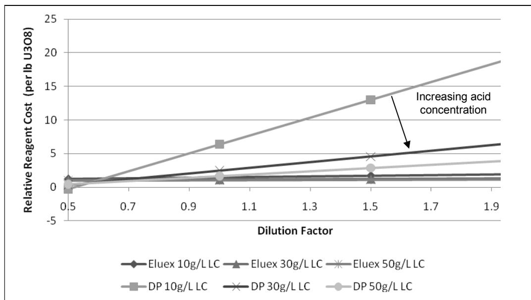
**Figure 8: Relative reagent costs with changing acid concentration (50g/L U<sub>3</sub>O<sub>8</sub> resin loading)**
