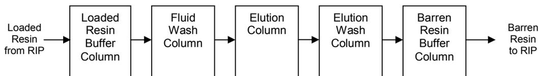
**Figure 2: Block flow diagram of continuous U-column elution**
