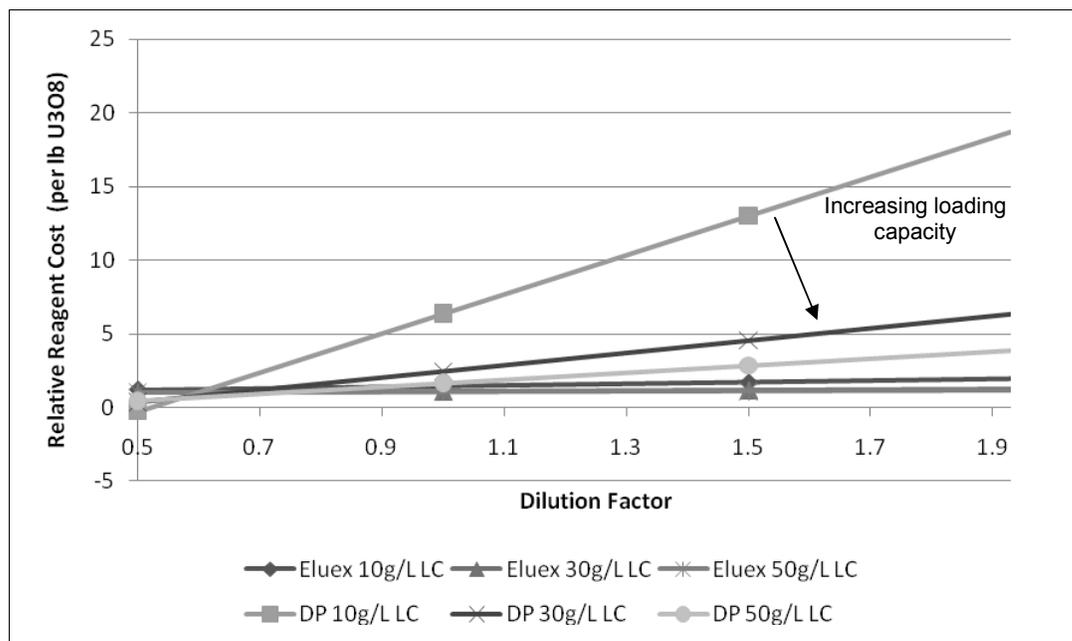
**Figure 9: Relative reagent cost with changing uranium loading (150g/L H<sub>2</sub>SO<sub>4</sub> in eluent)**
