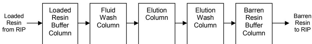
**Figure 1: Block flow diagram of continuous straight elution**
