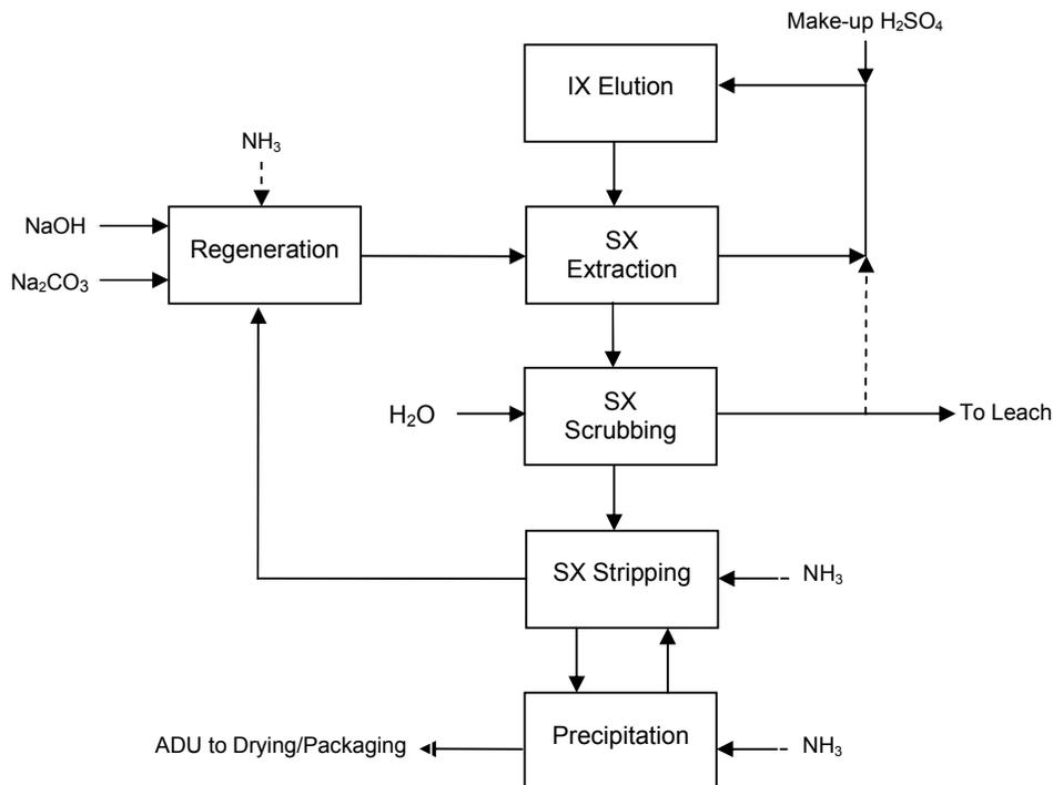
**Figure 7: Typical Eluex flow sheet**
