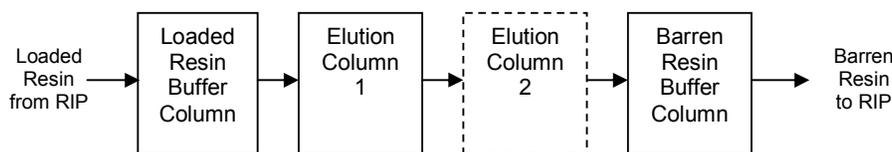
**Figure 5: Block flow diagram of NIMCIX elution**
