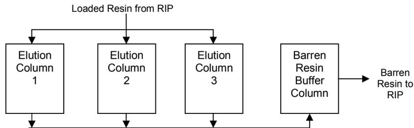
**Figure 4: Block flow diagram of Carousel elution**
